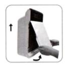
Pull the front panel and extract upward.
